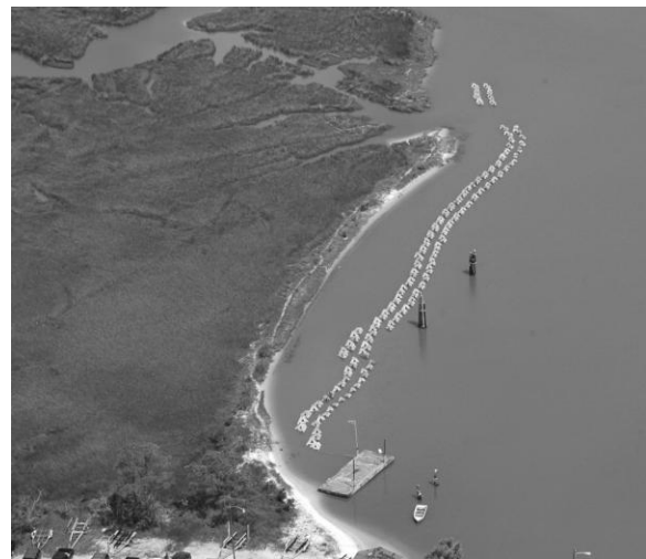
Figure 4. Aerial photograph of Saw Grass Point Salt Marsh, Pass Drury Channel, Fort Gaines Harbor, and the 182 coastal havens after they were installed. A visible gap between the long and short segments can be seen in front of one of the three tidal creeks within the marsh.
